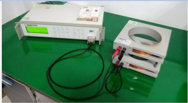
German Magnet-PHYSIK. Magnetic moment detection instrument (ELECTRONIC FLUXMETER EF5)
