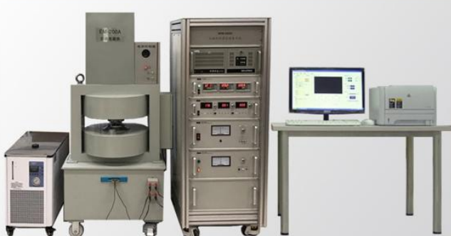
China Metrology Institute-double electromagnet high temperature permanent magnet measuring instrument NIM62000TA
