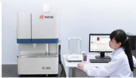
China Steel Research nano CS-2800 high frequency infrared carbon sulfur analyzer
